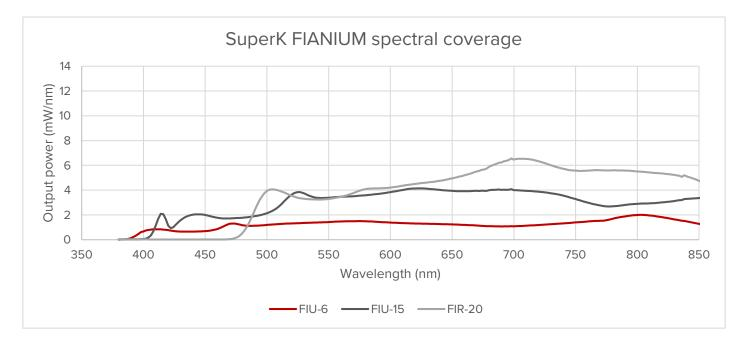
Visible power density curve of the high power lasers.
